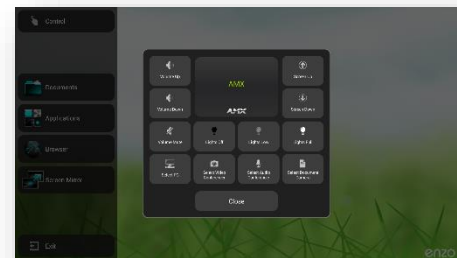
Enzo can be used to control audio, video and lighting in the room (separate AMX NetLinx Controller required)
